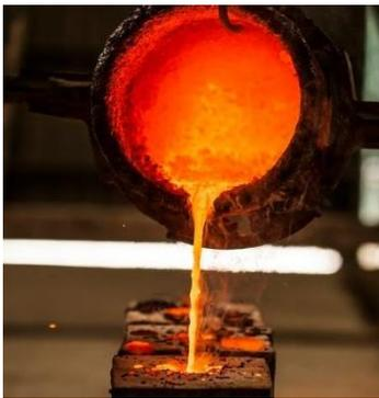
**Development of Oxygen-free High Strength Electrical Copper Alloy:** Addition of suitable alloying element in copper to ensure complete solid solubility followed by rapid quenching. Treating the melt with a suitable mix of de-oxidizers to prevent loss of alloying elements. Further 60-90% cold reduction to impart strength, followed by aging treatment to improve electrical conductivity to about 91-93% IACS.
